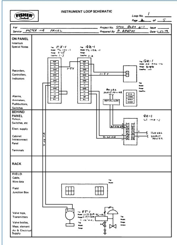
Figure 3. Example of a shop drawing. Loop diagrams must be generated from the P&ID.
