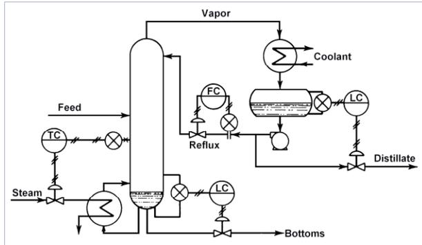
Figure 2. Example of a P&ID depicting two level loops, one temperature loop and one flow control loop. The SI is required to make submittals and shop drawings for these devices before purchasing and installing the equipment.
