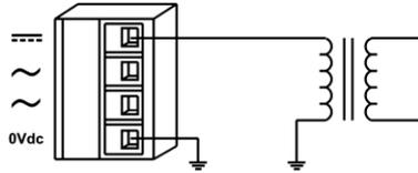
**Figure 5 — AC Powered with Grounded Secondary**
