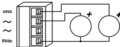
*Figure 3 — Redundant DC Powered*
