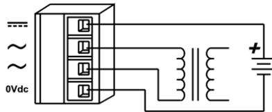
**Figure 6 — AC Powered with Battery Backup**
