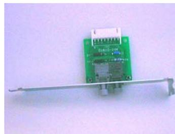
To complement the OCB mounted on the PA10 controller, an additional OCB was provided by Mitsubishi. It is a small board with a slot bracket (right image above). The remaining text describes how this board can be connected to a PCI22-485X. (The PA10 manual *Instruction Manual for Servo Driver* describes a similar retro-fitting for ARCNET cards equipped with an HYC4000 transceiver.)
