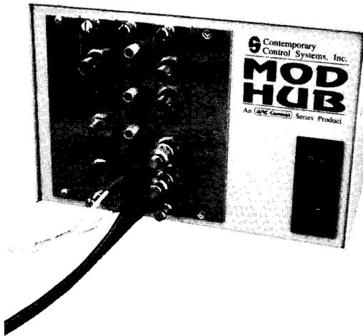
*Expansion modules are inserted into a MODHUB modular active hub. Cabling media can be mixed within one hub by selecting the appropriate EXP expansion modules.*
